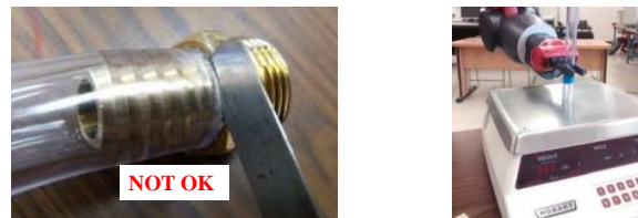
Figure 3: Measurement of quality of joint (NOT OK) and Measuring force exerted by CoBot
